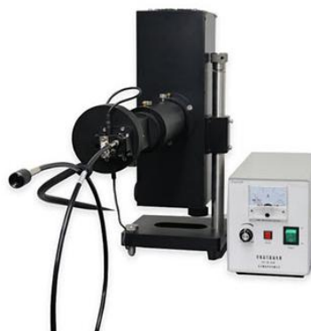
Mercury lamp 200-650 nm wavelength range
